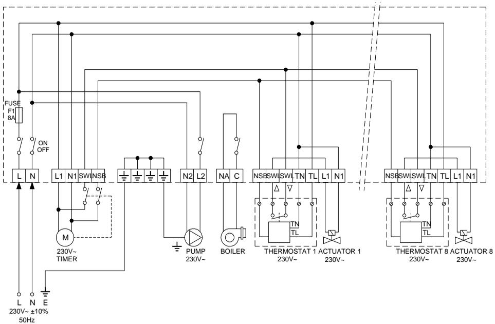
Fig. 4: Wiring diagram.
