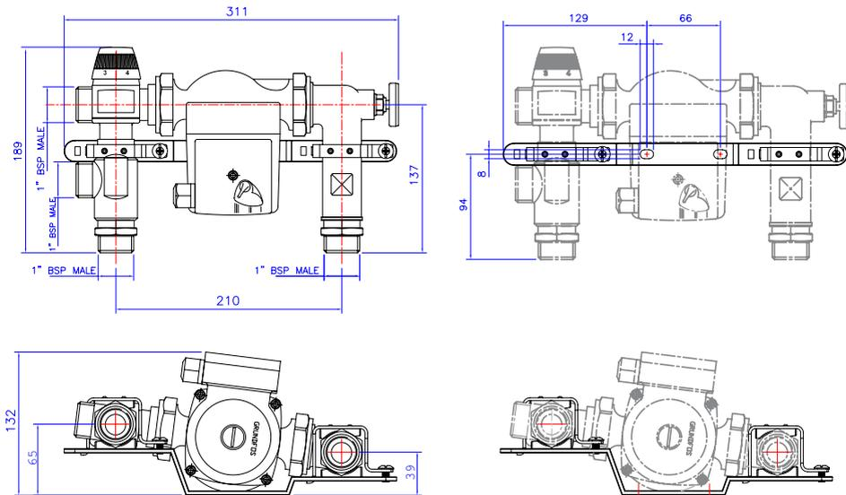
Fig. 1 Overall Connections and Dimensions
